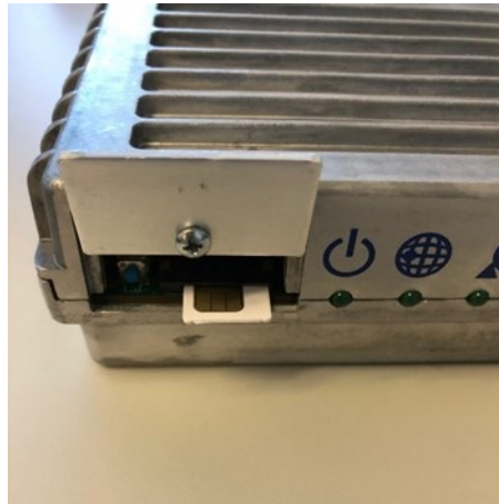
Figure 32: Installing the SIM card
