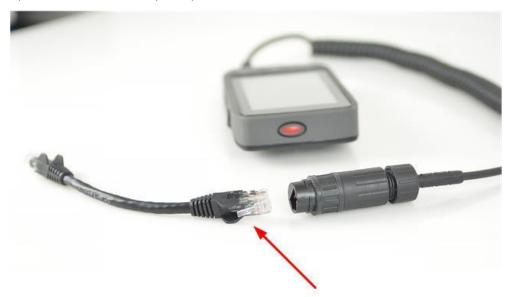
Connect Ethernet Cable to end of Coil Cable
