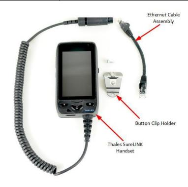
Figure 1-1 Thales SureLINK Handset Kit Components
