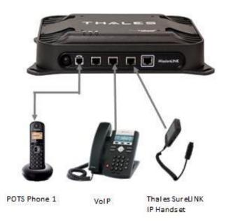
Figure 2-3 Thales SureLINK Handset Connected to TU/BDU
