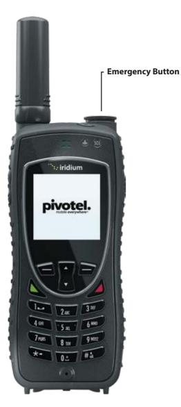
Dimensions: Weight: Operating Temp: Shock Rating: Dust Rating: Waterproof Rating: Battery Type: Battery Life: 140 x 60 x 27 mm 247 g -10 °C to 55 °C MIL-STD 810F IP6X (Dust Resistant) IPX5 (Water Resistant) Lithium-ion Talk-time: Up to 4 hours Stand-by: Up to 30 hours
